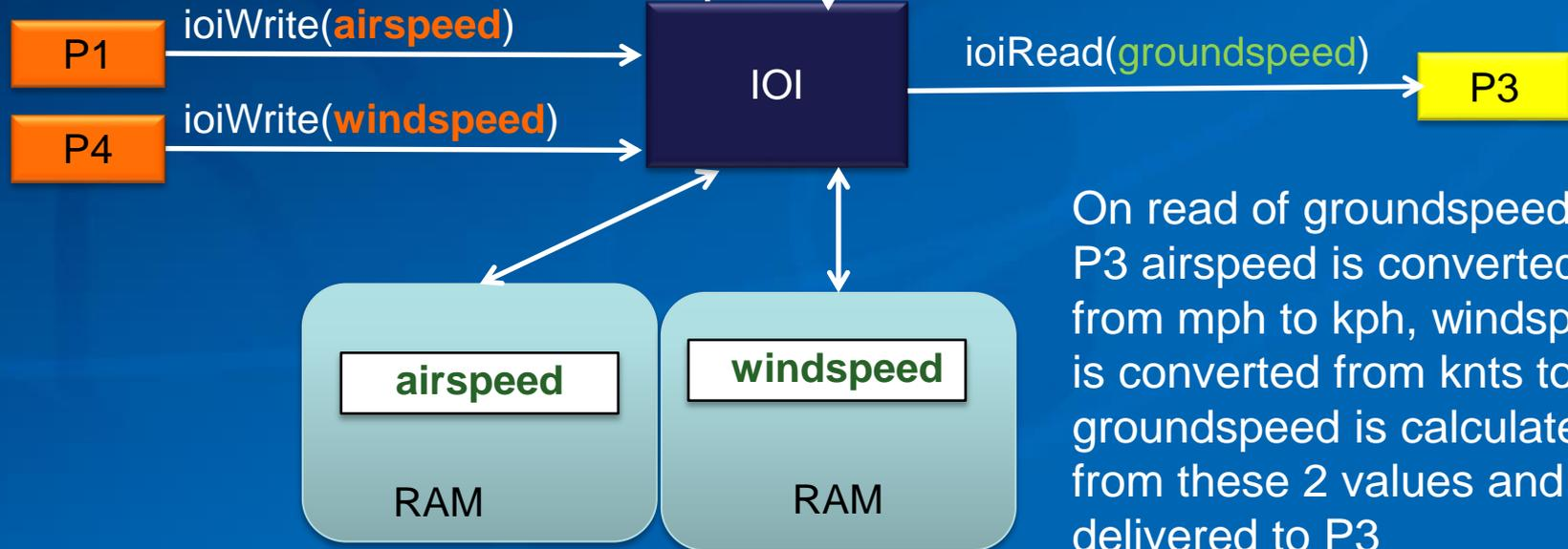
On read of groundspeed by P3 airspeed is converted from mph to kph, windspeed is converted from knts to kph, groundspeed is calculated from these 2 values and delivered to P3
