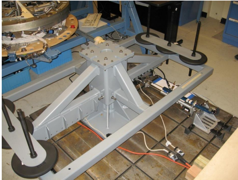
Rotational Mass Emulator (RME) Commercial Linear EMA Bench Test Step Input Test #052 (Compensated Controller Gains, High Load State (18 x 25 lbm Plates)) Test Executed: Dec 15, 2010
